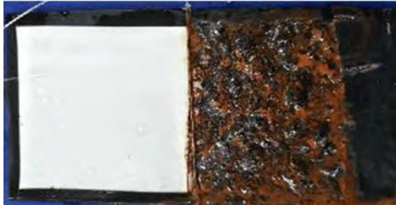
Left: TrueEco Nano Zinc-rich Paint + Nano Topcoat applied to carbon steel, after 2,000 hours of salt spray testing.
